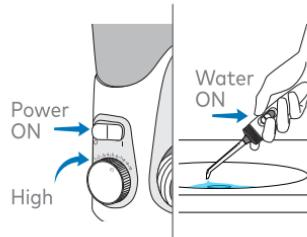
Turn pressure to high, point tip into sink. Turn Power switch ON and water switch ON until water flows. Turn OFF.
