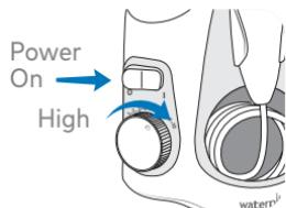
Turn pressure to High, point tip into sink, turn power and water switches ON until water flows. Turn switches OFF.
